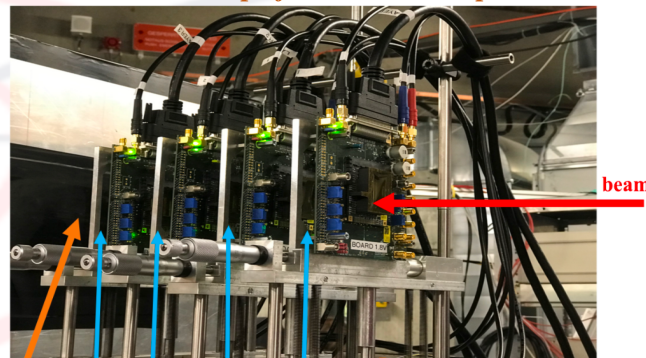
2-classical scintillators L3 L2 L1 L0 (DUT)
