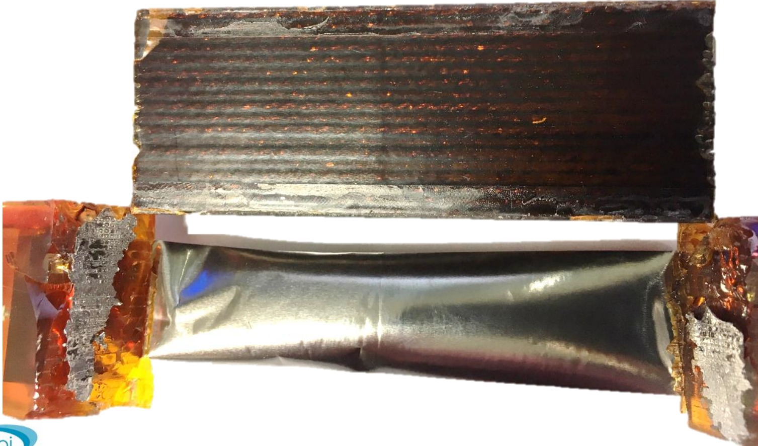
Sample with peeled off quench heater after cryogenic cycle to 1.9 K.
