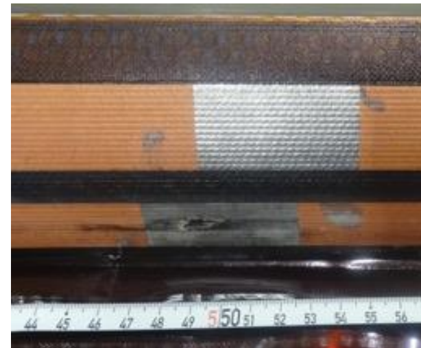
Type of direct short defect created in extended Hi-pot test on CR07, ( hole diam 2 mm, dumped E tot > 1kJ)
