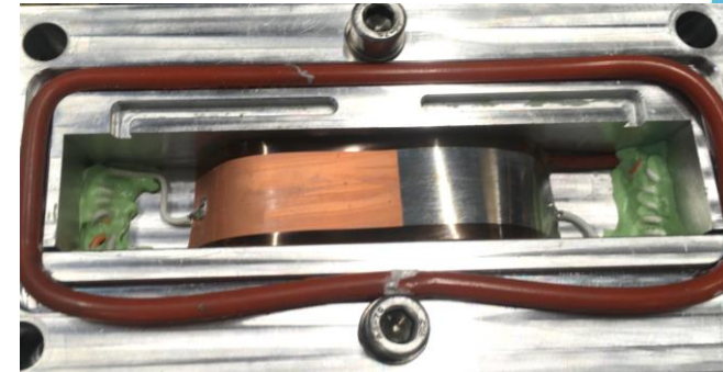
Prepared sample in the impregnation mould which enables radial and transversal compression
