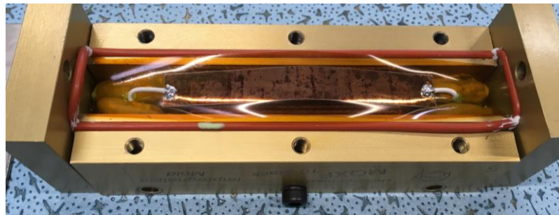
Impregnation mould for the investigation of the MQXF impregnation system.
