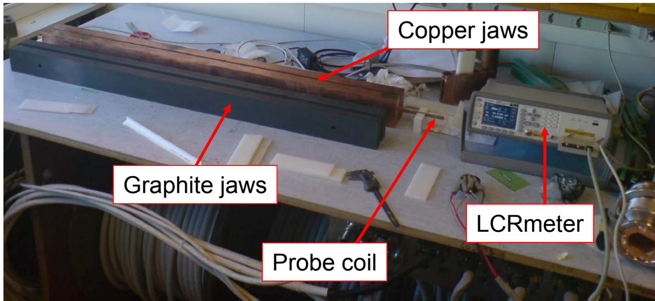
The electrical impedance of the coil  $Z_{\text{coil}}$  can be linked to the transverse dipolar beam impedance of the device  $Z_T$
