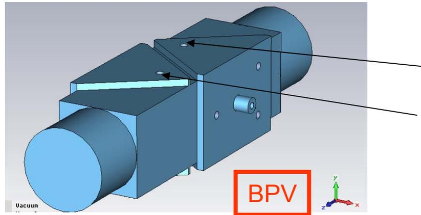
Ceramic insulator spacers designed to mechanically stabilize the thin electrodes
