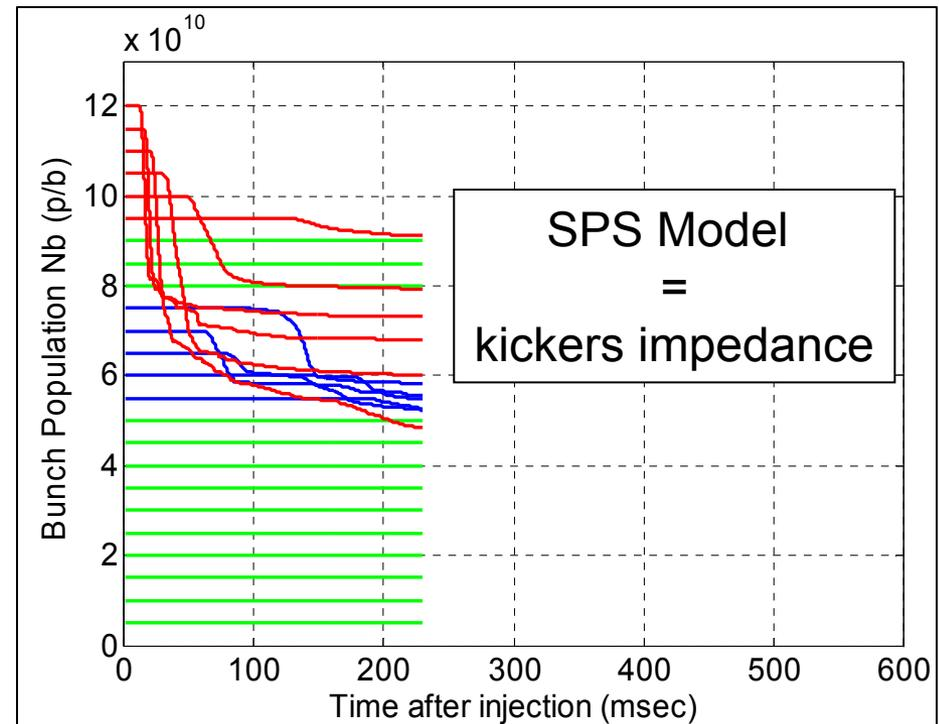
→ Similar pattern of beam losses between simulations and experiments
