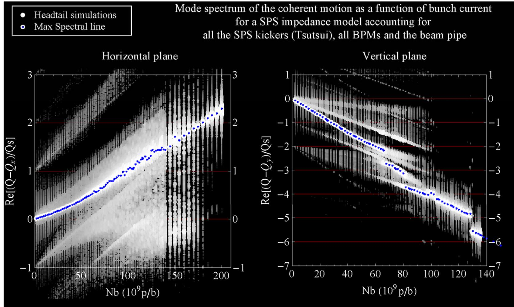
→ positive horizontal tune shift, as observed in SPS beam measurements since many years!
