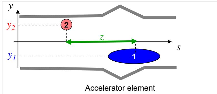
In general, we assume we can expand the wake anywhere in a transverse cross section with powers of  $x$  and  $y$
