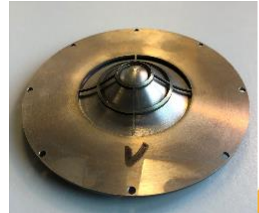
Tungsten prototype for heat load tests
