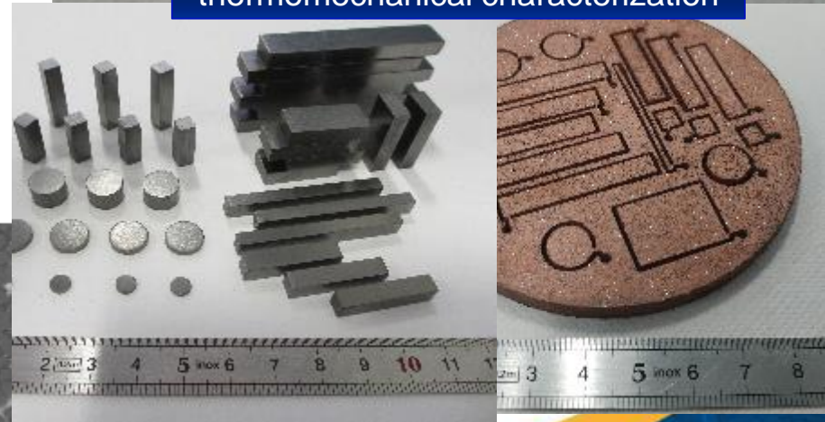
MoGr and CuCD samples for thermomechanical characterization
