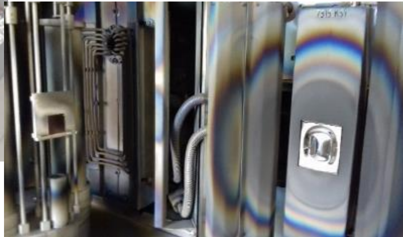
A sample during the Nb deposition at ASTeC/STFC
