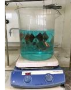
SUBU and Electropolishing treatments Courtesy of Crisrian Pira (INFN)
