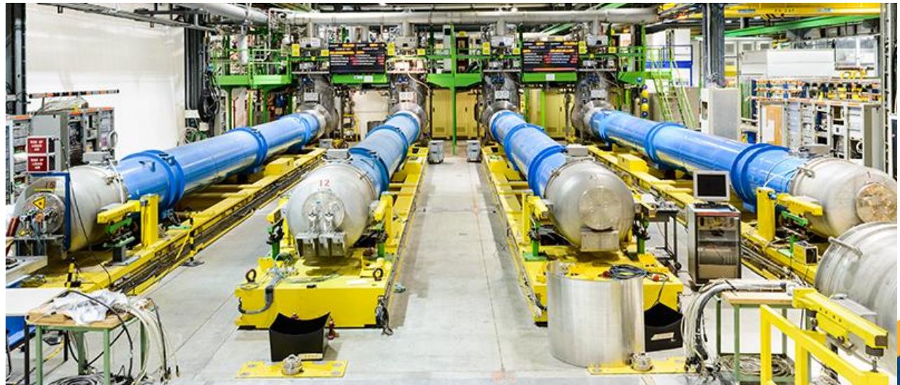
The CERN superconducting magnet test stand
