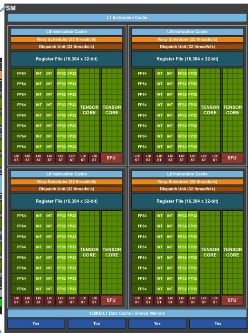
Figure 5. Volta GV100 Streaming Multiprocessor (SM)
