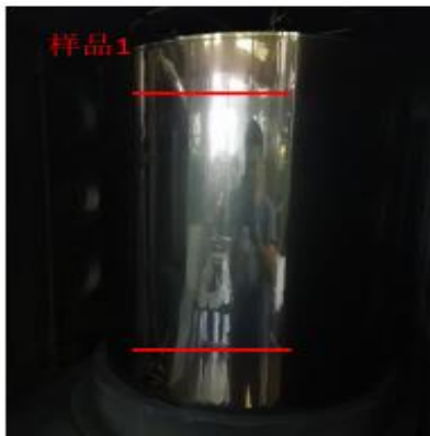
Large area DLC sample (1.2m \times 0.6m)
