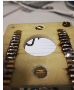
Multiwire Proportional Chamber(MWPC)
