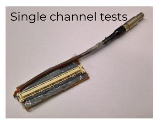
Pulses send to HRS connector directly pluged to hybrid
