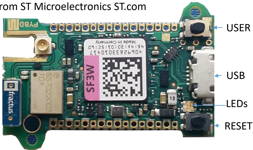
Top side with USB and Wifi antenna
