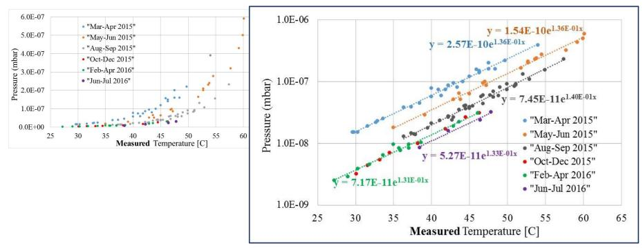
Since LS1 there have been periods of significant vacuum pressure rise in the MKP-L. The high pressure results in an important increase in the electrical breakdown rate. However:
