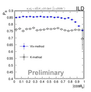
P<sub>B</sub> limited by vertex reconstruction efficiency, Particle ID efficiency and B0 oscillations.
