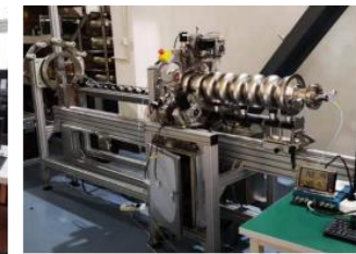
9-cell cavity pre-tuning machine
