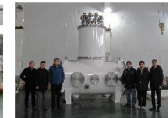
Horizontal test cryostat
