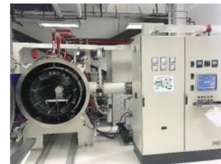
Vacuum furnace (doping & annealing)
