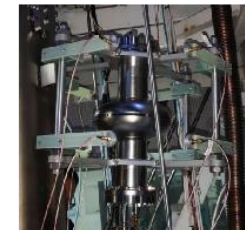
Second sound cavity quench detection system
