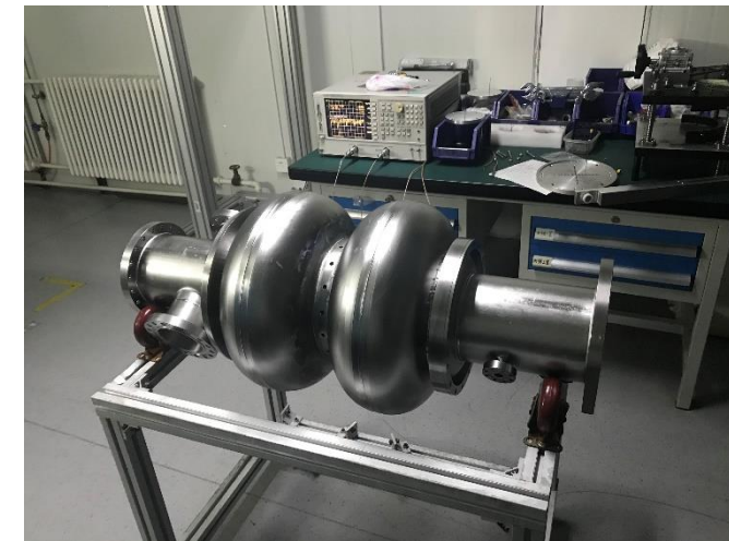
Collider ring 650MHz 2 cell cavity
