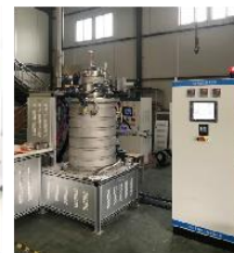
Nb 3 Sn furnace
