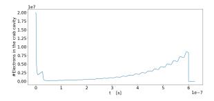
The electrons are pushed by the cavity with an energy that doesn't allow multipacting, therefore most of them are absorbed by the wall during the first RF period. On the other hand, some electrons are pushed to the adjacent drifts giving raise to multipacting in there.
