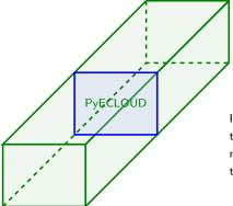
In this case, we can reasonably compare the PyECLOUD 2D simulation with the middle section of the Warp 3D simulation.
