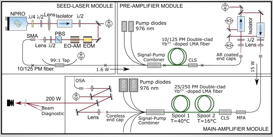
new design with reduced number of splices, reduced reflectivity and higher optical isolation
