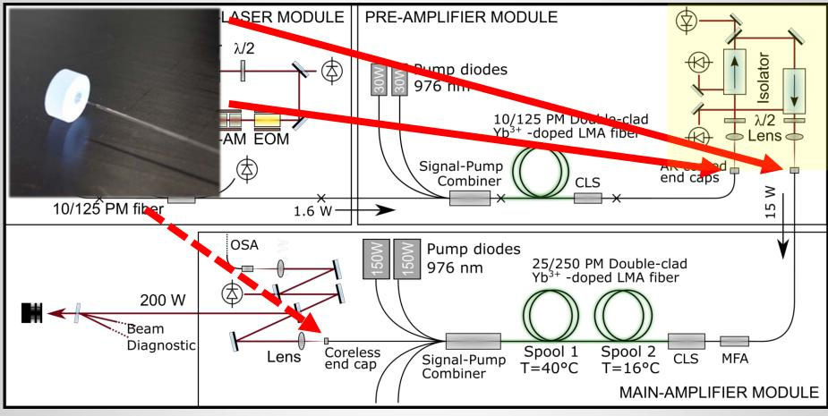
use AR coated fused-silica substrates at fiber-air interface in high-power FI unit and at high power output port
