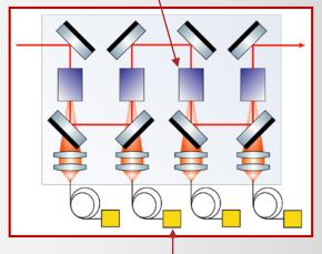
4 x 60 W Pump Diodes at 878 nm
