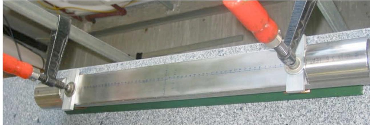
Pocket prototype constructed at Louvain and undergoing simulation and wire-testing at Cockcroft Institute for trapped modes, beam stability etc.
