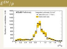
Ratio of EM energy in narrow window around impact cell and momentum of leading track for tau candidates identified as electron candidates Yann Coadou (CPPM) — Taus in ATLAS
