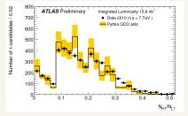
Ratio of high threshold to low threshold hits in the transition radiation tracker for tau candidates identified as electron candidates
