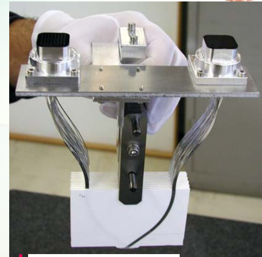
scintillator plate for triggering
