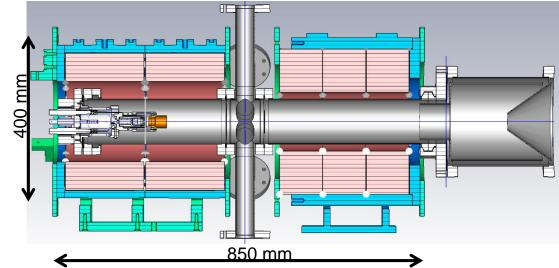
Parameters of the E-lens test stand :
