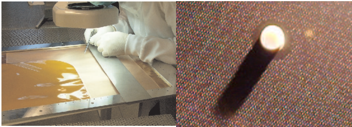
Figure 6.12: left: Positioning of the spacers in the clean room. right: A single spacer glued onto the GEM foil on the especially intended copper spot.
