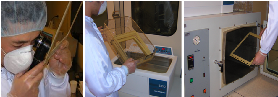
Figure 4.15: The clean procedure of the frame. From the left to the right: the visual inspection; the cleaning in the ultrasonic bath; the drying in the oven at 80 °C.
