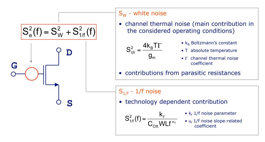
White and 1/f noise have been measured on test devices with different geometries and biased at different drain currents
