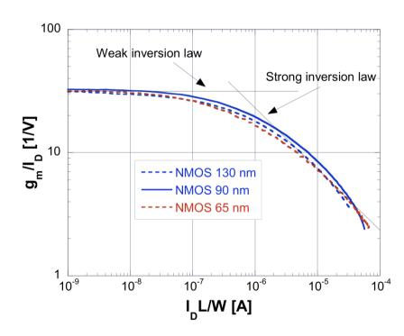
At a given drain current, operation is shifted towards weak inversion region with technology scaling
