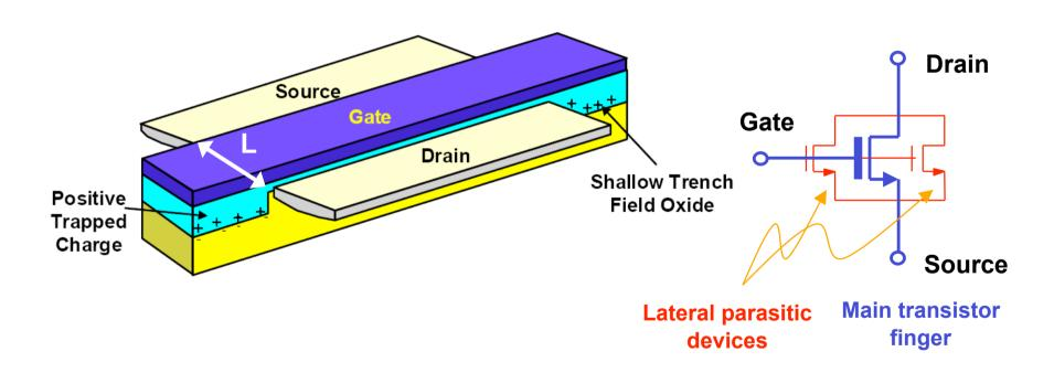
Radiation-induced positive charge trapped in isolation oxides may invert a P -type region in the well/substrate of NMOSFETs creating a leakage path between source and drain
