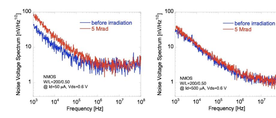
Moderate 1/f noise increase at low current density, due to the contribution of lateral parasitic devices
