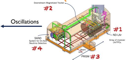
System for moving the LArTPC and tracker up to 30m transverse to the beam
