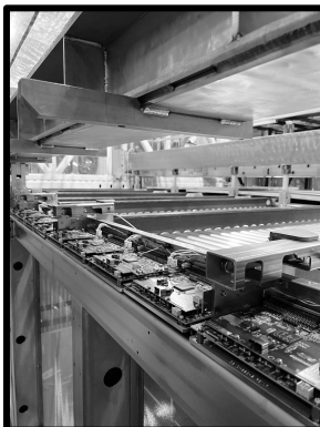
Photon Detection System boxes fully installed behind anode wire planes, September 2022
