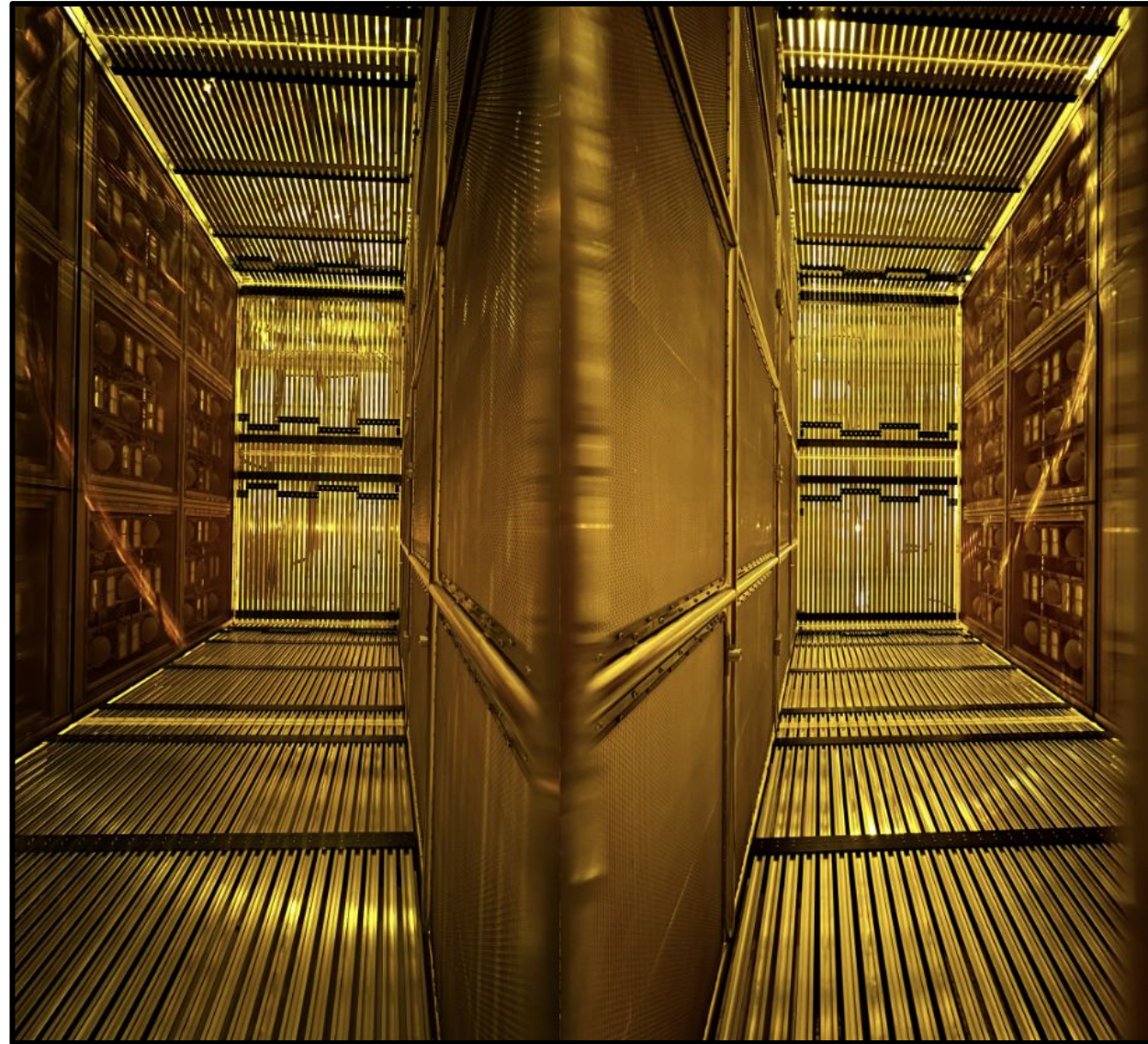
Fully completed assembly of 2 TPCS + Photon Detection System, September 2022
