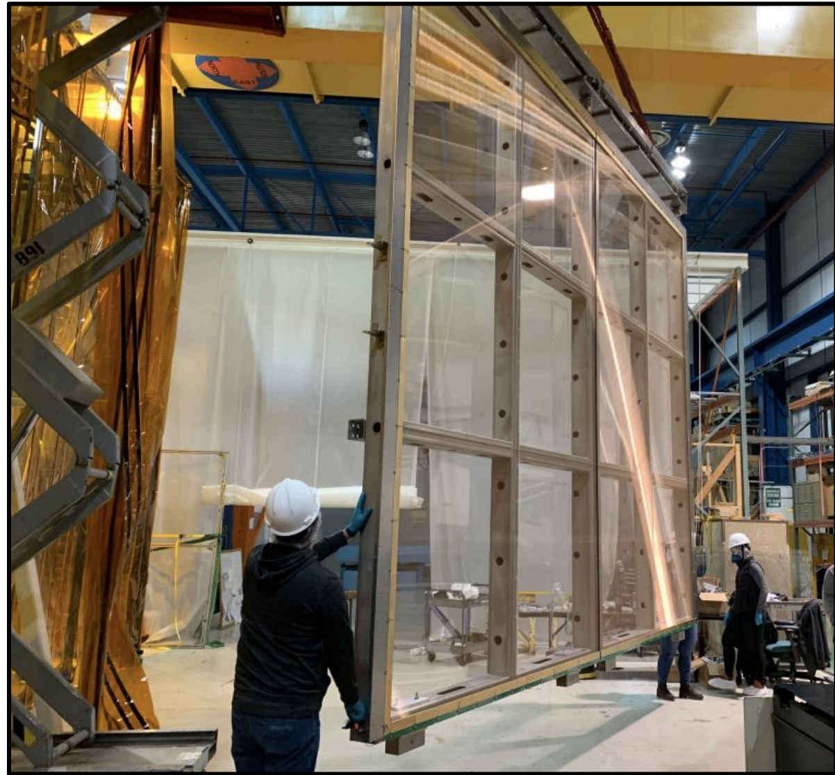
Anode Plane Assembly with wires being brought into place, October 2021
