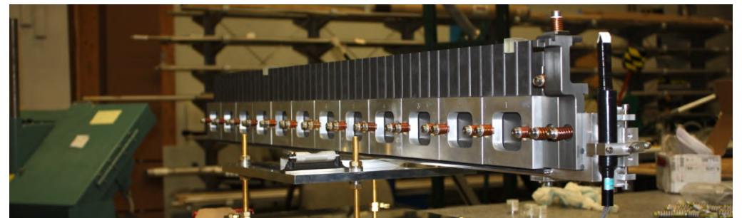
NuMI replica graphite target (120 cm, 2.5 \lambda )
