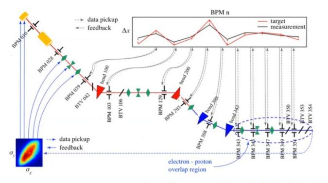
Tuning 15 components simultaneously: 2 solenoids, 3 quads, 10 steering magnets to simultaneously maintain the desired orbit and minimize emittance growth,
