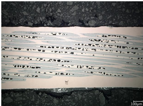
Figure 11 a) The location of the cracks is shifted from the middle of the sample, , b) Magnified view of 11a), cracks in the Nb 3 Sn phase
