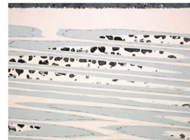
Figure 5 – a) Magnified view of the stitched image, crack in the Nb 3 Sn phase – b) Centre of the sample, no crack observed – c) Magnified view of 5b)
