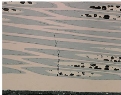
Figure 5 – a) Magnified view of the stitched image, crack in the Nb 3 Sn phase – b) Centre of the sample, no crack observed – c) Magnified view of 5b)
