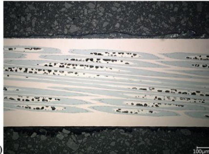
Figure 5 – a) Magnified view of the stitched image, crack in the Nb 3 Sn phase – b) Centre of the sample, no crack observed – c) Magnified view of 5b)
