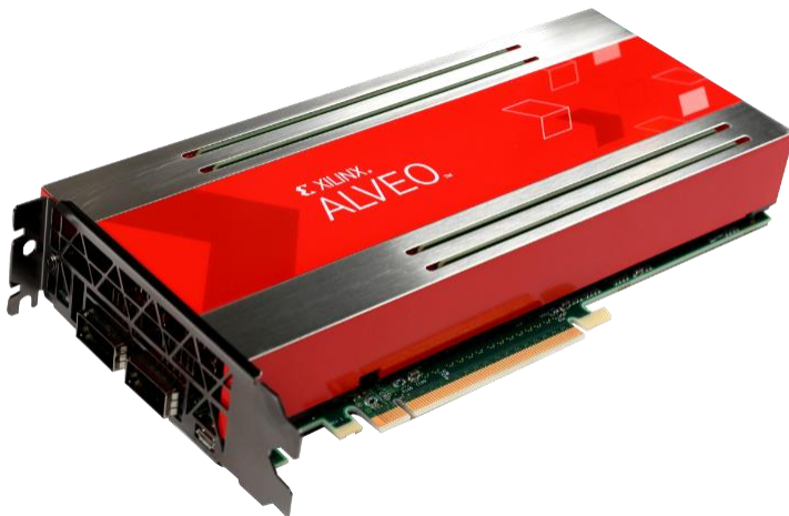
4x Xilinx Alveo U250 Accelerator Cards High-end FPGA (Xilinx UltraScale) based accelerator card with 2x QSFP28, PCIe Gen3 x16, 64GB DRAM@77GB/s, 57MB SRAM@47TB/s per card
