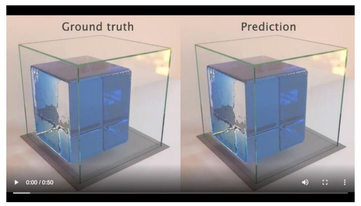
The time lap shows properly simulated water volume evolution (left) and simulated evolution by the trained neural network (right) with "Graph Network-based Simulators".
