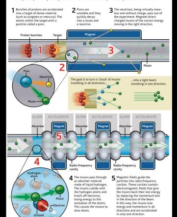
This process is repeated until the muon beam is almost laser-like, ready for injection into the main accelerator.
