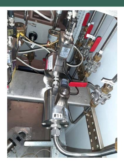
Closed leak on the R134a MFC in the RPC mixer
