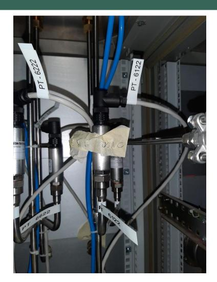
Leak on the PT – 6122 is over the scale of the instrument ( > 9999 ppm)
