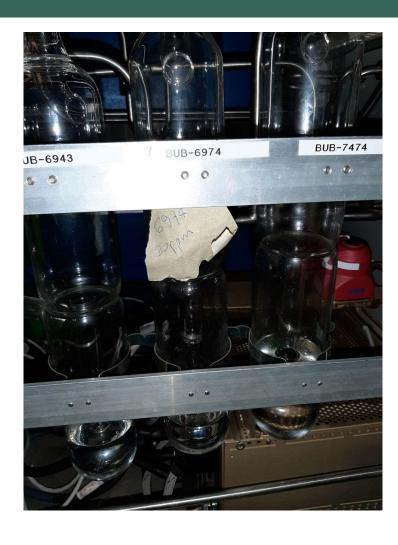
Leak on the safety bubbler 6974 is 400 ppm
