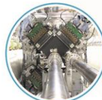
BEAM GAS VERTEX Two new novel beam instruments based on beam gas vertex detectors will allow non-invasive accurate measurements of the beam size.
