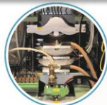
CLIQ A novel concept of magnet protection, based on fast injection of oscillating currents, will improve the safety of the very large stored energy quadrupoles.
