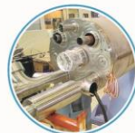
QUADRUPOLE MAGNETS 24 new quadrupole magnets of 11.4 tesla peak field, based on advanced Nb 3 Sn superconductor, to double beam focusing at ATLAS and CMS collision points.
