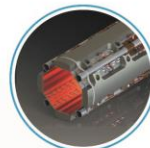
BEAM SCREEN All new magnets will be equipped with a new special beam screen to intercept collision debris at 60 K temperature and cancel electron-cloud effects.
