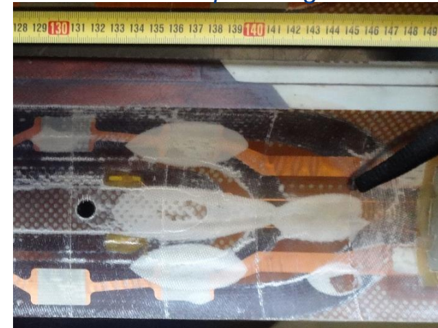
Inner layer heater in a MQXF coil after coil powering
