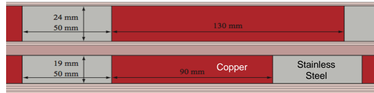
Outer layer heater design
