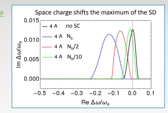
LHC injecton,E = 450 GeVBunch intensity: $N_b = 1.15 \times 10^{11} \text{ p}$ Linear SC param.: $\Delta_0 = -1.1 \times 10^{-3}$
