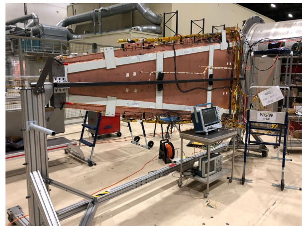
Figure 9: Small sTGC Wedge with Oscilloscope Connected
