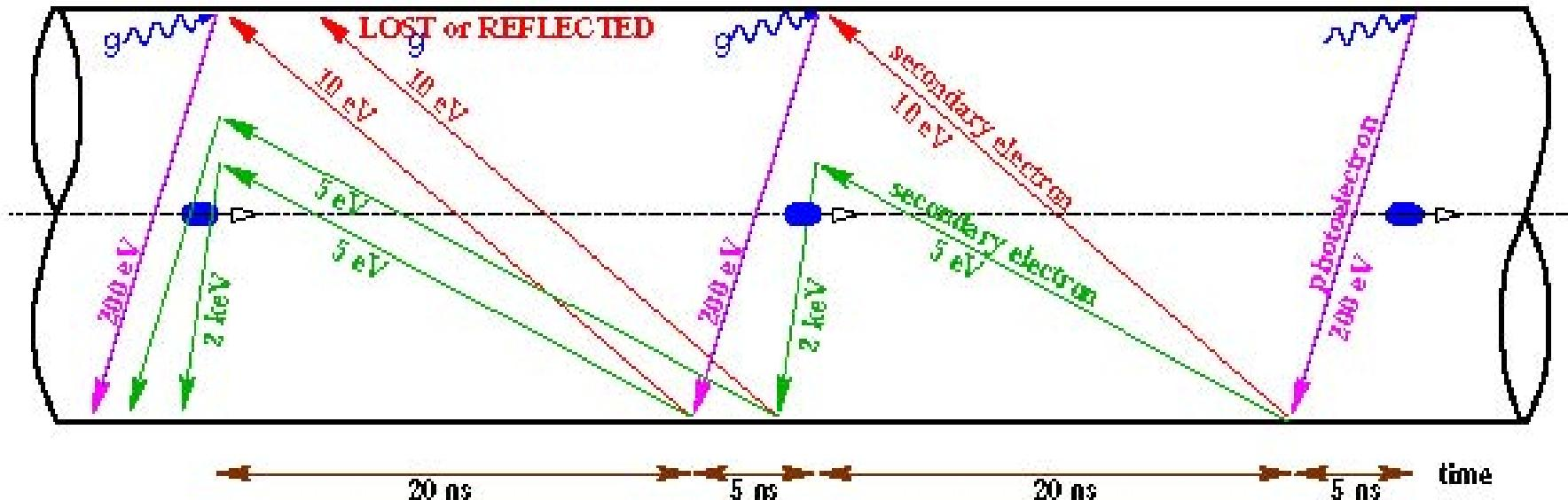
schematic of e- cloud build up in the arc beam pipe,
