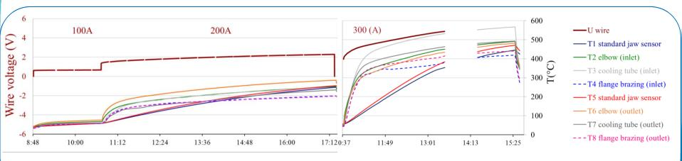
Tests performed on spare wire-in-jaw, under vacuum with no coolant
