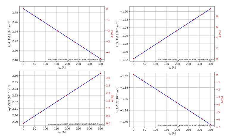
When we trim a wire the Q4/5 close to the wire are trimmed to compensate as close as possible the quadrupolar perturbation of the wire.
