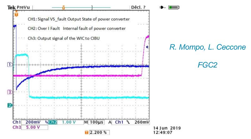
Confirm (*M. Zerlauth*) WIC path sufficient interlock chain even for the most (time) critical failures of the wire compensator
