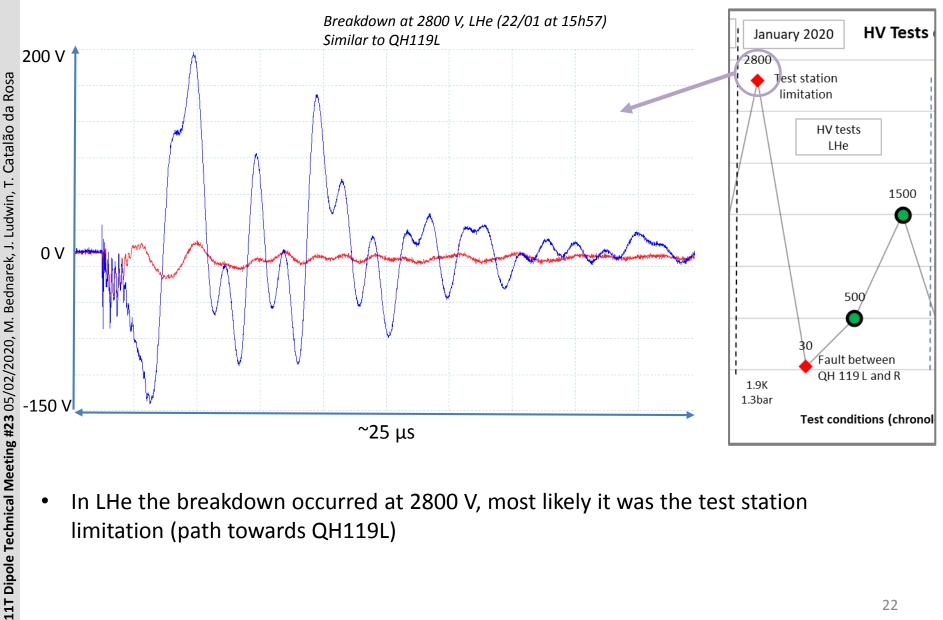
In LHe the breakdown occurred at 2800 V, most likely it was the test station limitation (path towards QH119L)
