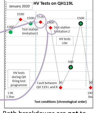
Both breakdowns are **not** to the magnet circuit
