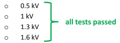
Insulation was tested up to 1.6 kV without current before final provoked quench.
