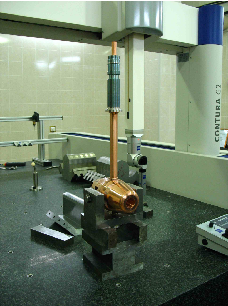
Inclination due to EBW is 4'
