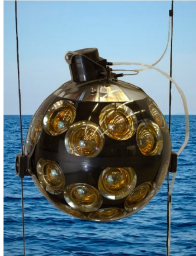
1 optical module = 31 photomultiplier tubes
