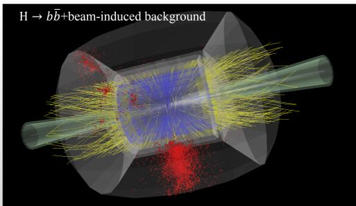
$\mu^+\mu^- \to H\nu\bar{\nu} \to b\bar{b}\nu\bar{\nu}$  + beam-induced background fully simulated
