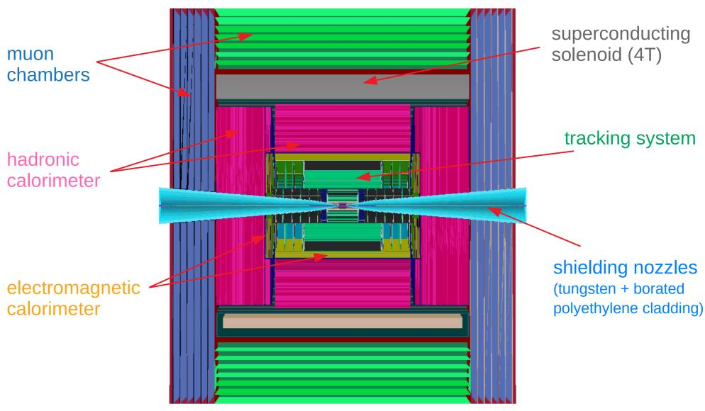
This is basically CLIC's detector + the shielding nozzles.
