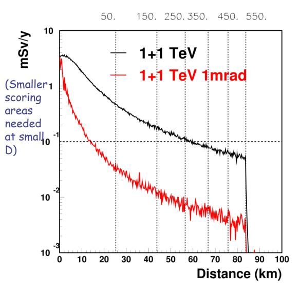
Dose vs distance from exit, or depth, for a straight section
