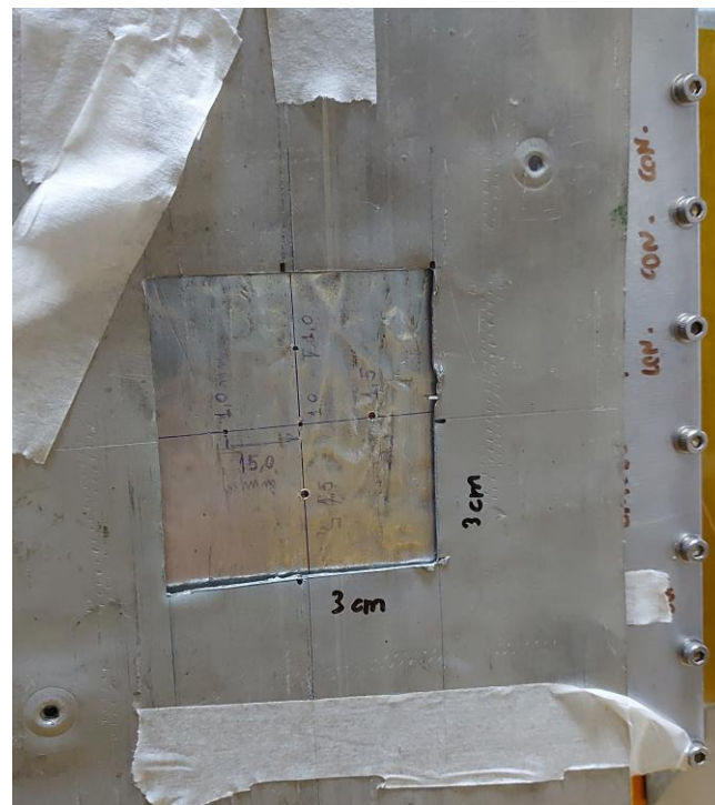
Left side: scan calibrated Cadmium mask. Center: mask over detector. Right side: obtained image (329062 events).
