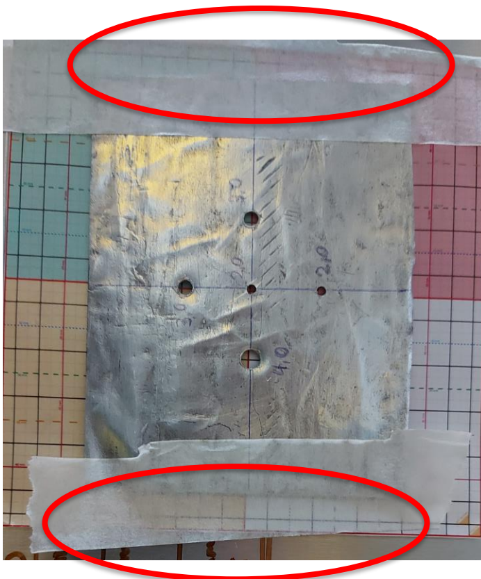
Left side: Mask over detector; the mask is smaller than the beam. Right side: obtained image (833311 events).
