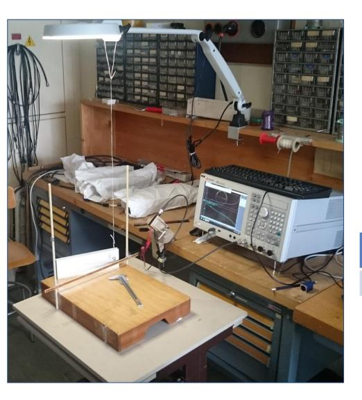
The measurements have been done with different blocks in different displacements. The chosen reference for them was the loop centre. It was mandatory to bear in mind that it was almost impossible to determine the loop centre without touching the loop itself.
