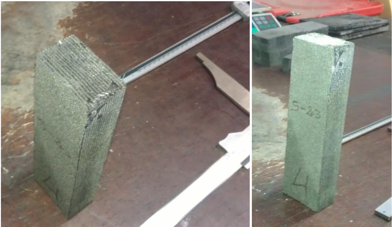
Picture 1, TCDQ block graphitized to 1.4g/cm 3 density.
