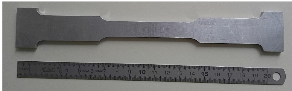
Sample geometry according to ISO 6892. Thickness: 4 mm
