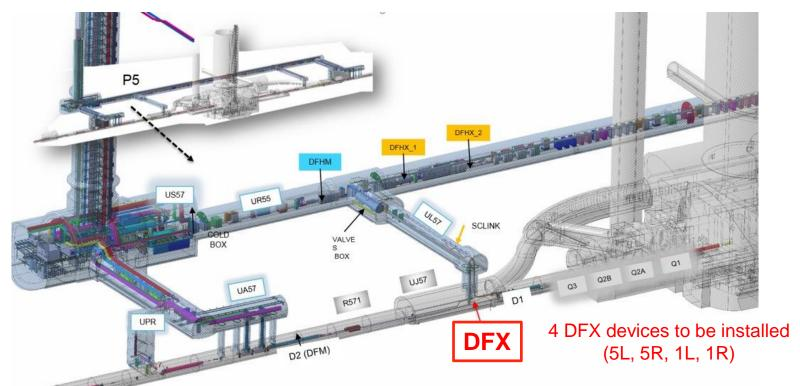
Interface between **SC Link** and **Diodes Cold Module** of the **HL-LHC Inner Triplets**
