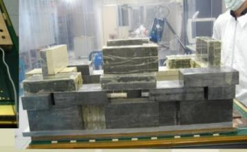
A heavy Al plate is placed to distribute the pressure
