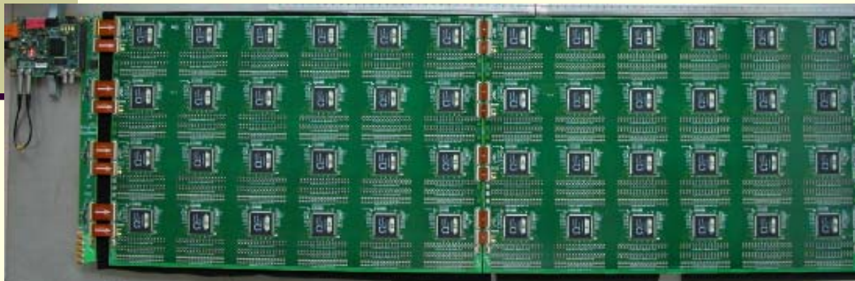
2 chained ASU of 32x48 cm 2 bulk with 24 HARDROC2
